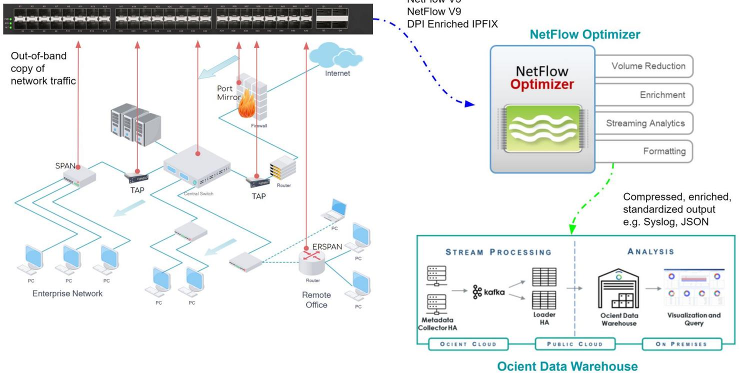
As in the example above combination of Cubro TAPs and mirror ports (such as SPAN and ERSPAN feeds) provide a copy of all network traffic to an Omnia120. The Omnia120 generates DPI enriched IPFIX records from all traffic sessions. These records are sent to a local instance of NetFlow Optimizer for processing, aggregation, and further data enrichment. The output is standardized and sent to a remote centralized installation of Ocient Data Warehouse for retention and analysis.
